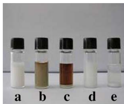
Figure 7 Chemical sensing by the single-crystalline nanoslabs: (a) ampoule containing a colloidal suspension of single-crystalline ZnO, which appears white; (b) the appearance of the ampoule (deep-brown suspension) after the addition of 4-triethoxysilylaniline (sample taken after 4 h of addition) and (c) the appearance of the ampoule (dark-brown solution) after sedimentation. (d) The appearance of the ampoule (white suspension) after the addition of 3-ethoxysilylpropylamine (sample taken after 4 h of addition) and (e) the appearance of the ampoule (semi-opaque white solution) after sedimentation.
